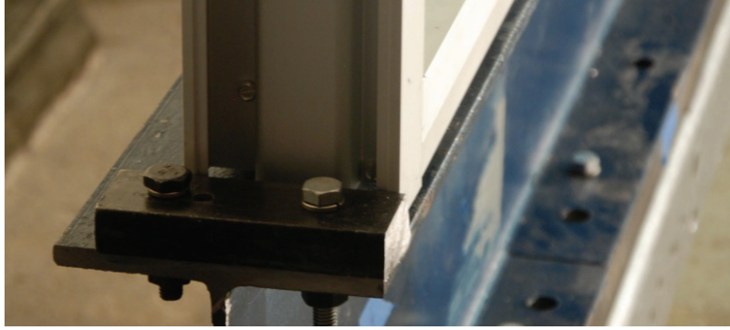
Figure 27: Example of an end restraint.
