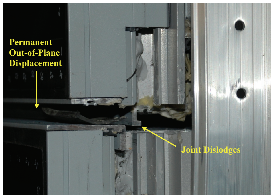
Figure 56: Dislodging of Horizontal Stack Joint and Lower Right Panel.
