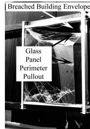
Figure 66: Laminated glass pullout behavior due to glass panel buckling shown here for a laminated glass unit.
