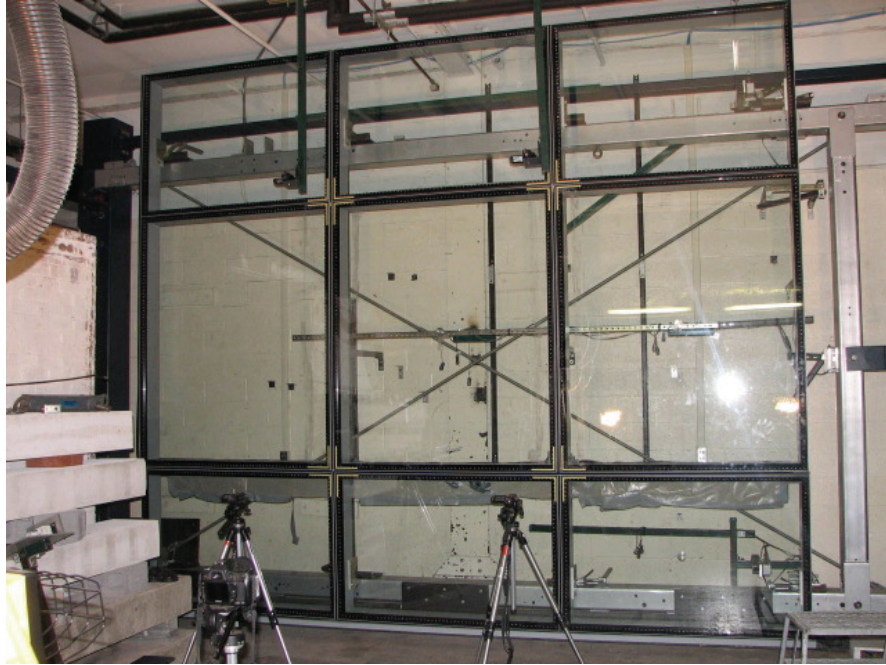
Figure 46: Fully Built Unitized System Test Specimen.
