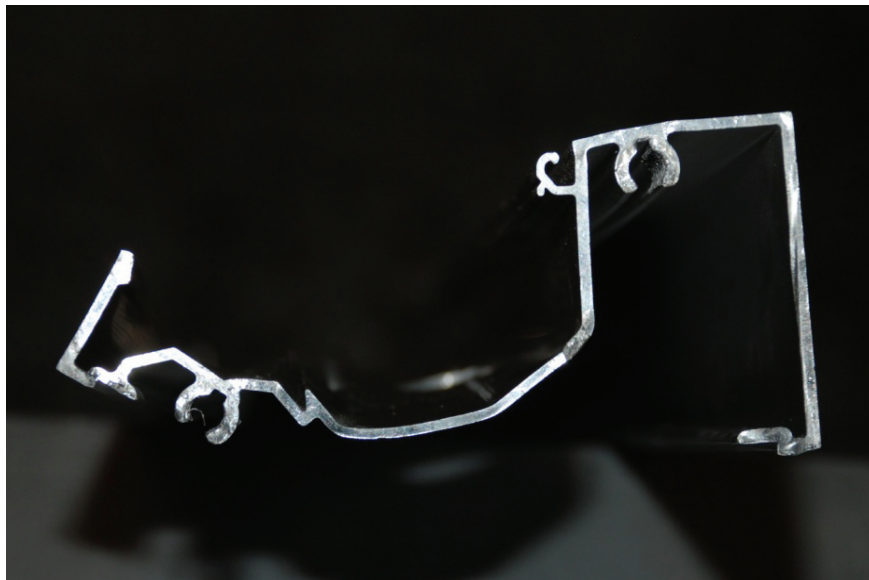
Figure 30: Typical damage to horizontal mullions.
