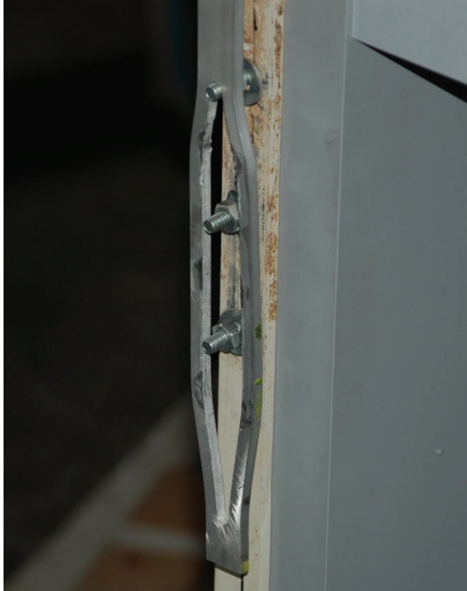
Figure 61: Extent of Slotted-Hole Widening.
