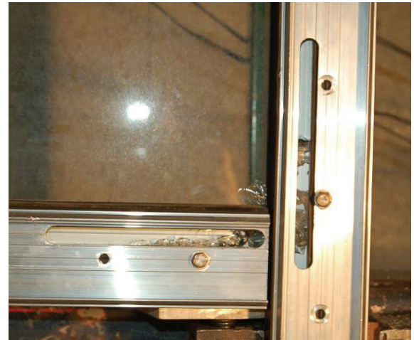
Figure 23: A test on an AN mono pane where viewing slots were created along the pressure plates at the corners so that localized glass corner crushing and spalling could be observed.
