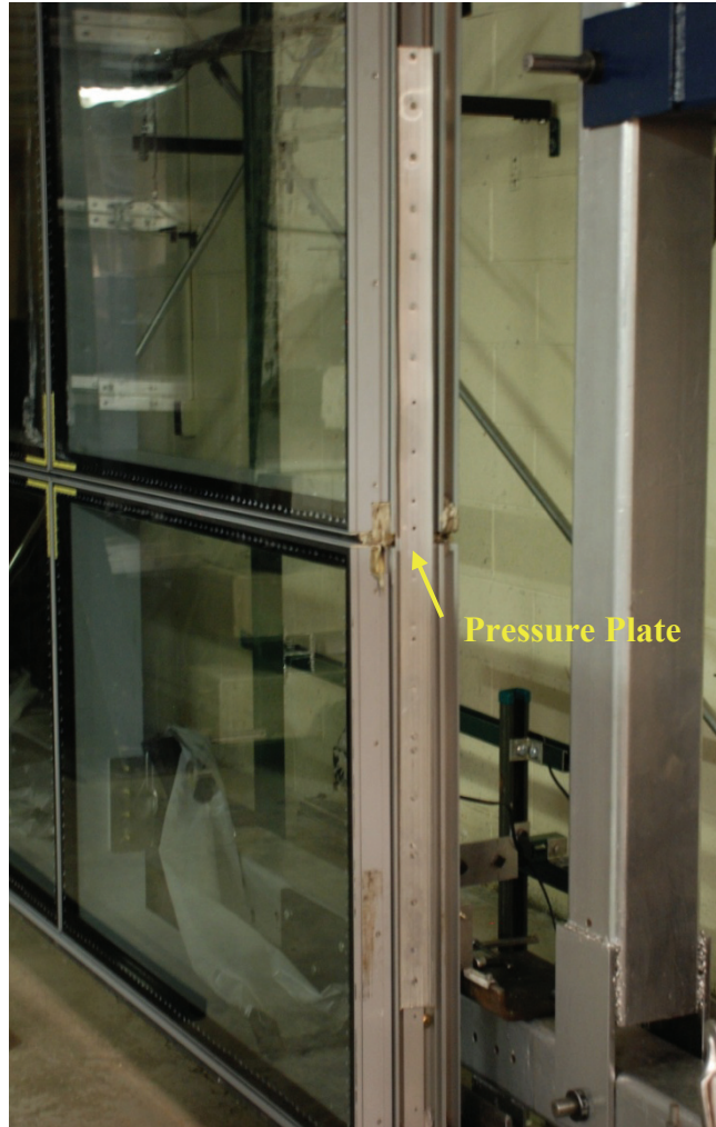
Figure 53: Pressure Plate Attached to First Specimen as an End Boundary Condition.
