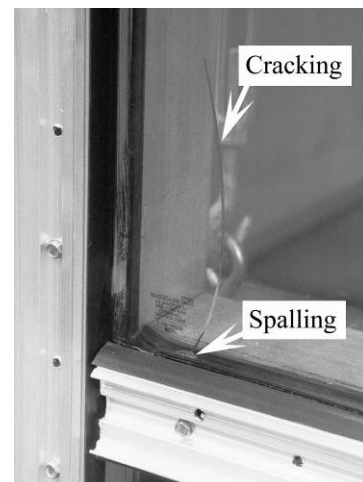
Figure 21: Glass cracking caused by localized corner crushing.
