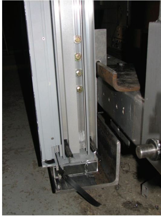
Figure 40: Attachment of the Bottom of the Specimen to the Facility.
