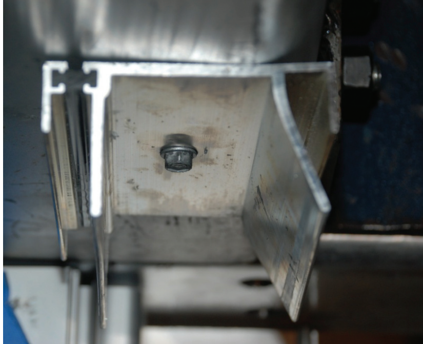
Figure 33: End of test condition of a reentrant corner head anchor.
