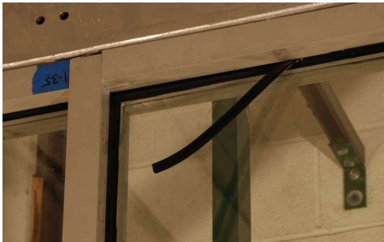
Figure 29: Gasket rolling (top), and gasket pullout (bot.).
