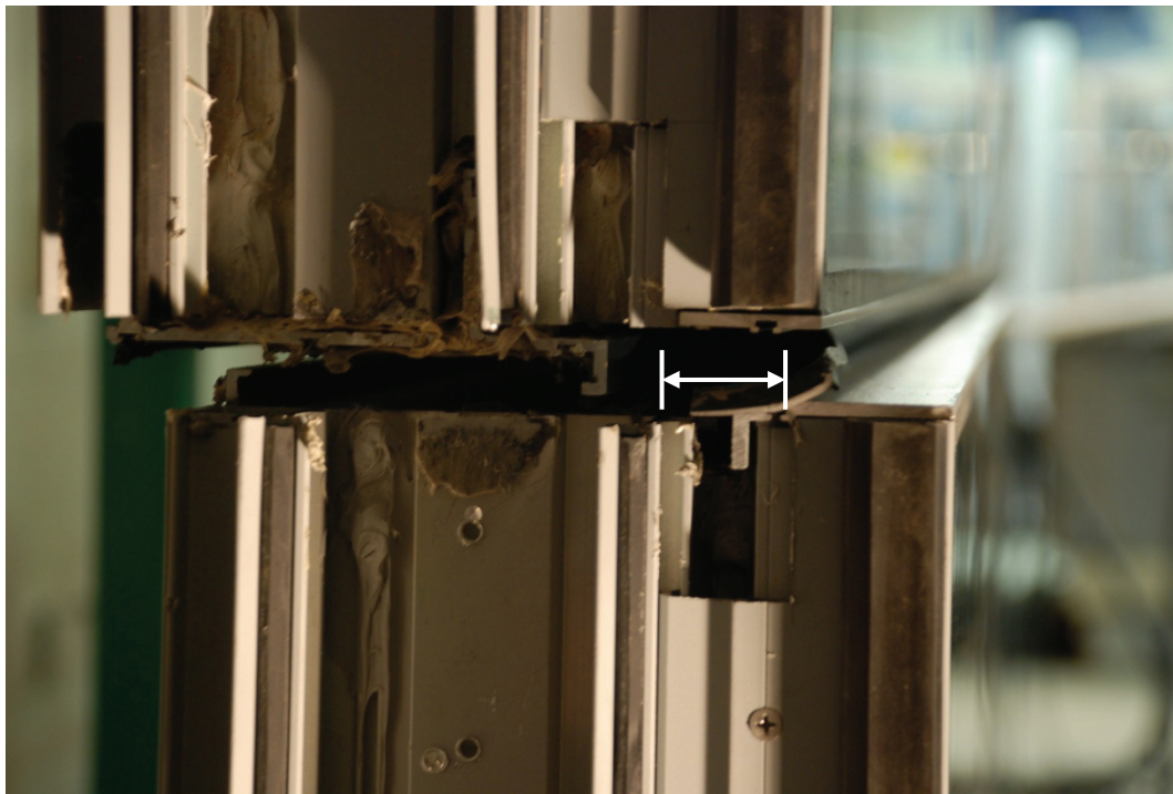
Figure 62: Horizontal Stack Joint Dislodges from Lower Left Panel (Magnitude is shown by arrow).
