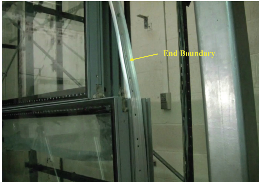
Figure 55: End Boundary Acting as a Tension Member.
